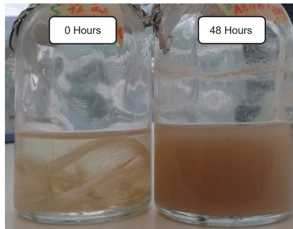
Figure 42. Hydrolysis of feathers after by consortium Azotf36 at the end of 48 hours enrichment passage 12.
