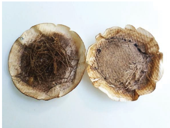
Figure 27. Substrate of lignocellulosic biomass (grass mixtures) filtered after 7 days of incubation at 60 °C. Inoculated with consortium Azotdp36 (right) and the negative control (left)
