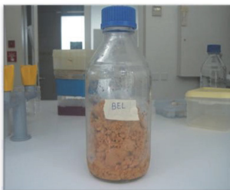
Figure 2. Glass containers with sewage sludge for sterilization and storage at 4 °C until use.
