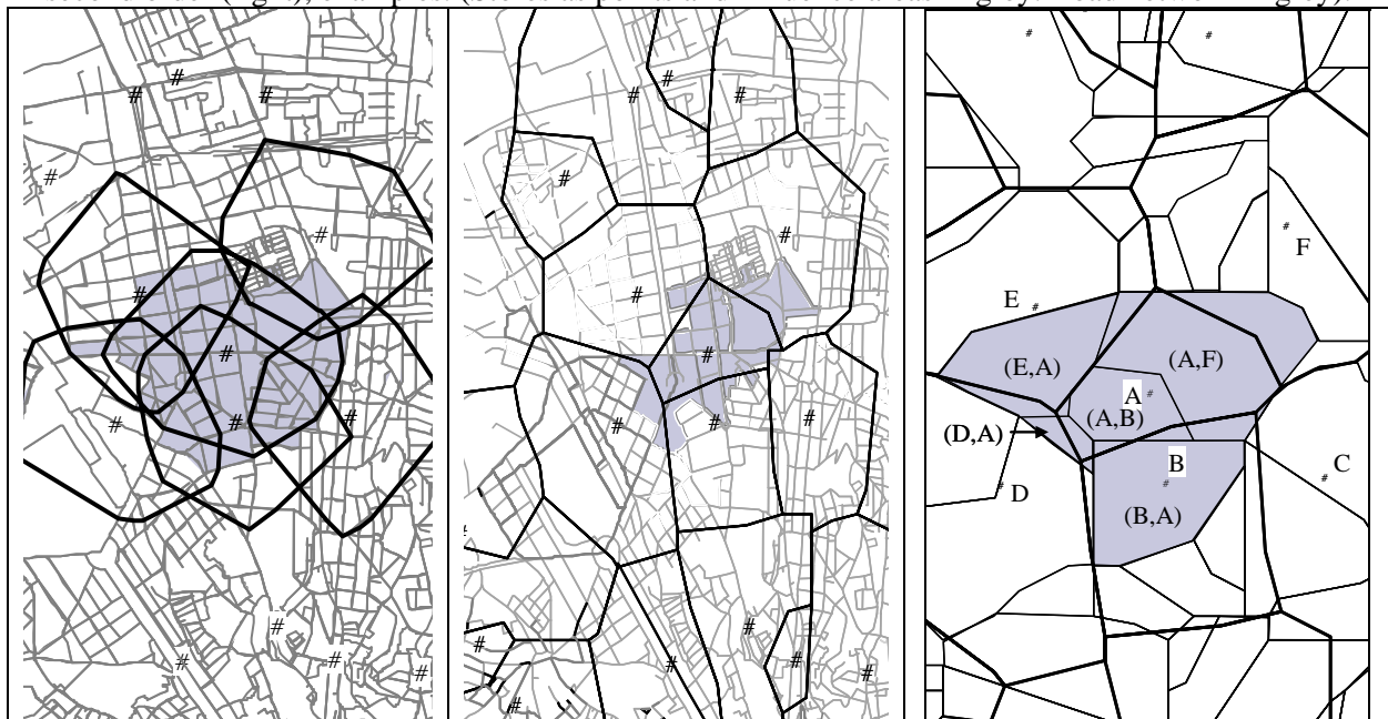
Figure 2. Shortest path polygons (left) and multiplicative weighted Voronoi diagrams, first (centre) and second order (right), examples. (Stores as points and influence areas in grey. Road network in grey).
