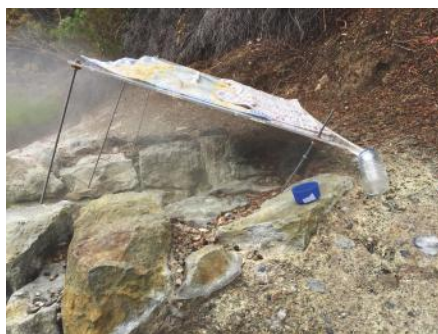
FIGURE 1. Fumarole Condensate collection in Furnas locality.
