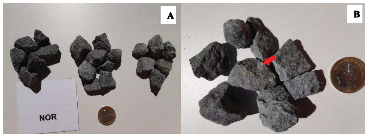
Figure 5.109. Macroscopic photos of the NOR aggregate with different fractions: A) General view; B) detail of one of the fractions with white areas (red arrow).
