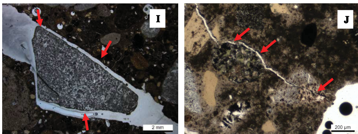
Figure 5.87 (continued). Photomicrographs of concrete prisms incorporating Icelandic aggregates. All photos are in PPL. I) Limestone aggregate particle debonded from the cement matrix (ICL4 sand); J) Crack starting in rhyolite aggregate particle and outlining other aggregate particles (ICL4 sand). The red arrows point to the cracks.
