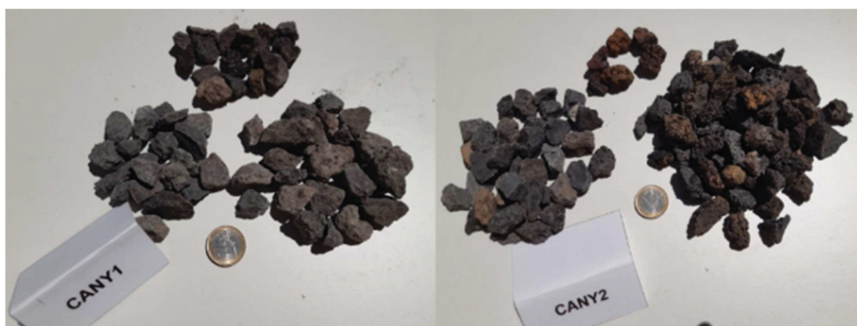
Figure 5.11. Canary samples of aggregate in crushed rock are split into different fractions according to the texture and colour.
