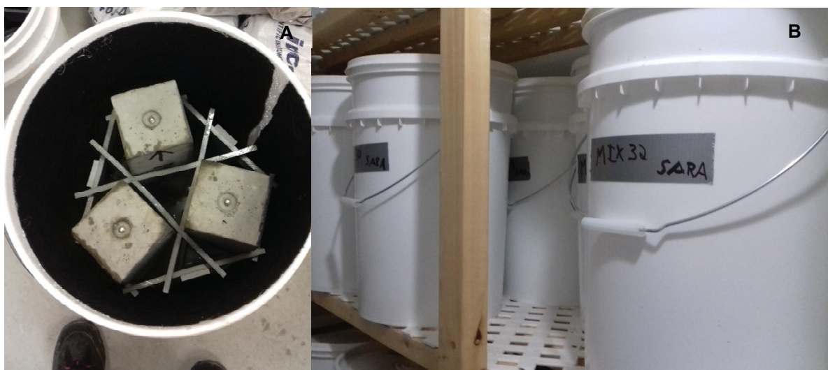
Figure 4.13. Plastic container /pails: A) with a wick and 3 prisms inside a rack; B) inside a chamber at 38°C.
