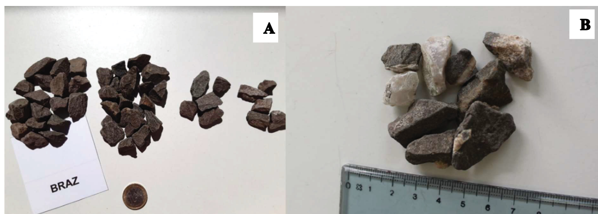
Figure 5.97. Macroscopic photos of the BRAZ aggregate divided in different fractions. A) General view; B) detail of the fraction with white particles.
