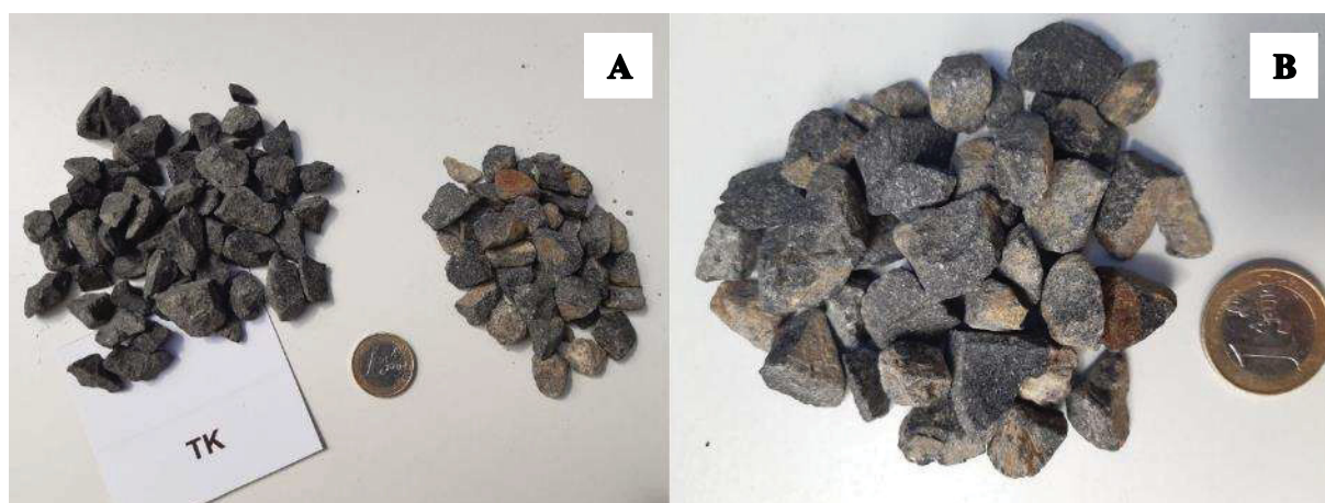
Figure 5.113. Macroscopic photos of the TK aggregate with different fractions: A) General view; B) detail of one of the fractions with white dots and the surfaces lined by a beige or red colour material.
