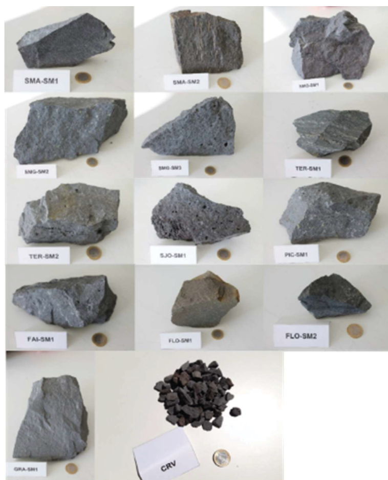
Figure 5.9. Block samples of the Azorean rocks were used as aggregates. Only the CRV sample is formed by crushed aggregate.
