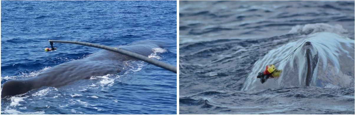
Figure 9: DTAG-deployment with a hand pole on a sperm whale (left) and a successfully attached DTAG on a sperm whale back (right). Photo credits: Mónica A. Silva @AzoresWhaleLab.
