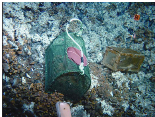
Fig. 4. Traps for macrobiological collection, e.g. shrimps, crabs and fishes. Photo: © ATOS - IFREMER
