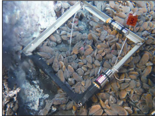
Fig. 3. Chemical sensors sampling a vent chimney at Lucky Strike vent field. Photo: © ATOS - IFREMER
