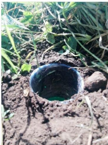
Figure 2. A pitfall trap. The trap was then covered with a plastic dish raised from the ground to avoid overflow of the trap due to eventual rainfall (Photo credit: Sophie Wallon).
