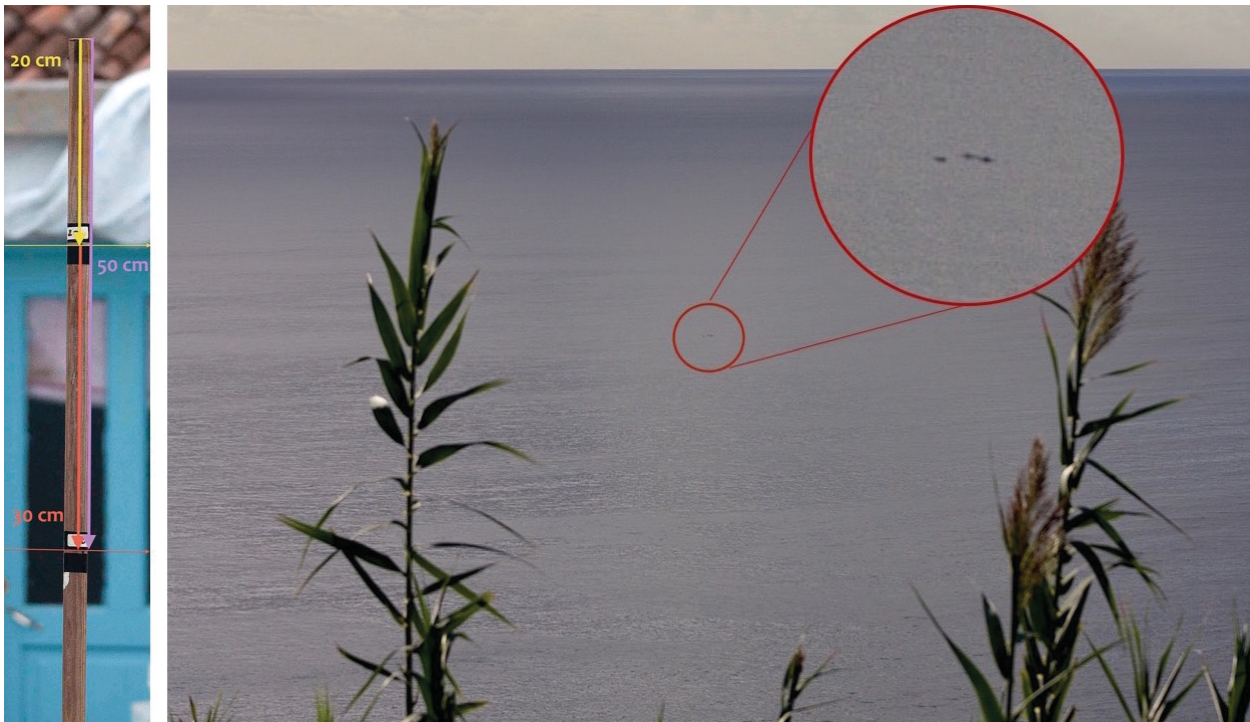
Figure 2.4 Stick used to calibrate the focal length of the camera during focal follows. Located at 5m distance from the stationary support, it shows three different measures accounting for camera adjustments (left). Example of camera shot during a focal follow (right).
