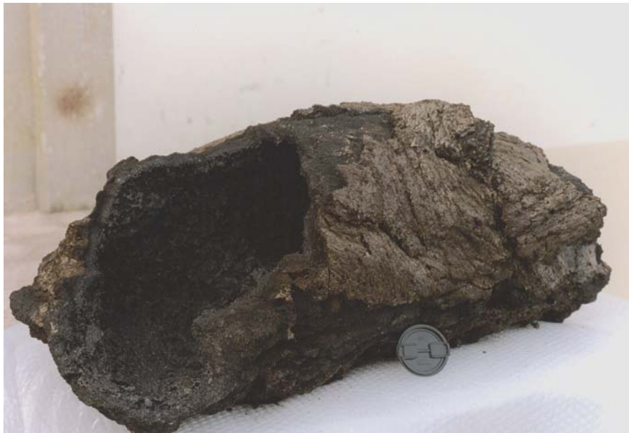
Foto 5.4 - Sample collected on February, 10. Note the void interior and the thin crust that prevented gas to escape.
