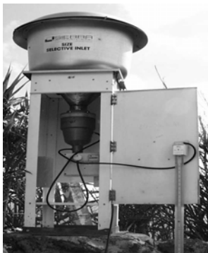
Figure 2a. High Volume Sierra-Andersen (model SSI 120) with a cascade impactor Tisch TE - 231F
