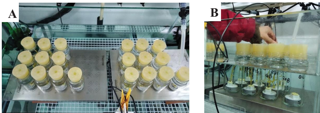
Figure 14: (A) Incubation system with magnetic stirring plate in water bath maintained with temperatures of 14 \pm 0.1 °C and 250ml glass chambers with rubber lids where the oxygen PSt3 sensor are read with the oxygen meter Fibox4; (B) O 2 measurement with the oxygen meter Fibox4.
