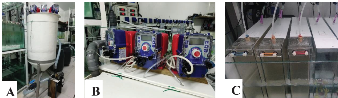
Figure 12: (A) reservoir 114L tank used to prepared sediment “stock”; (B) Dosing pumps that delivered sediments from the reservoir tank to each aquaria; (C) silicone tubes attached to the aquarium lids.
