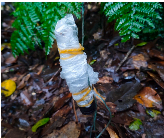
Fig. 2. Configuration of a data logger at ground level (GRD). Note the supplementary protection against adverse weather conditions. The sensor heads are positioned in a downward direction to prevent the accumulation of rain.
