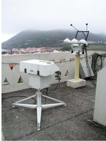
Fig. 1. Measuring radiation setup from AZONET (AZores Observation NETwork) at José Agostinho Observatory in Angra do Heroísmo: Brewer MKII spectrophotometer (left) and the sun tracking system setup (right).
