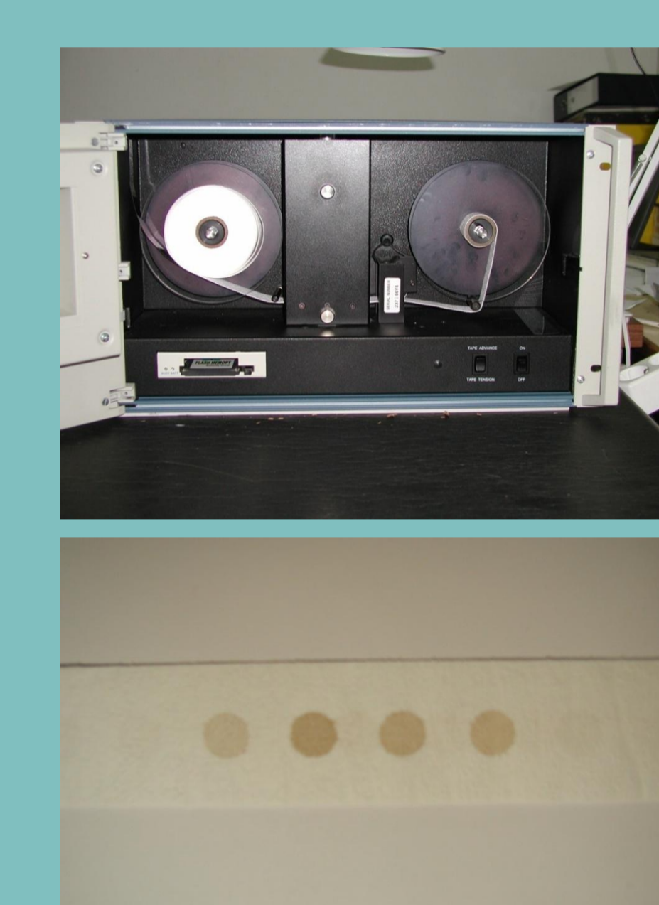
Fig 3. Instrumental set-up for the quartz-fibre filter tape on site and an exposed section of the tape after removal at the laboratory (four identifiable spots).
